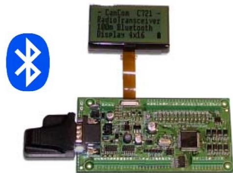
CanCom circuit board C721 for use in portable remote control devices.
