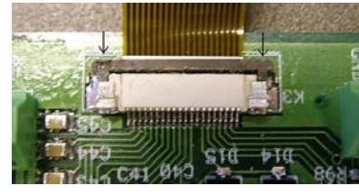
1. Turn the display cable according to the picture above.
