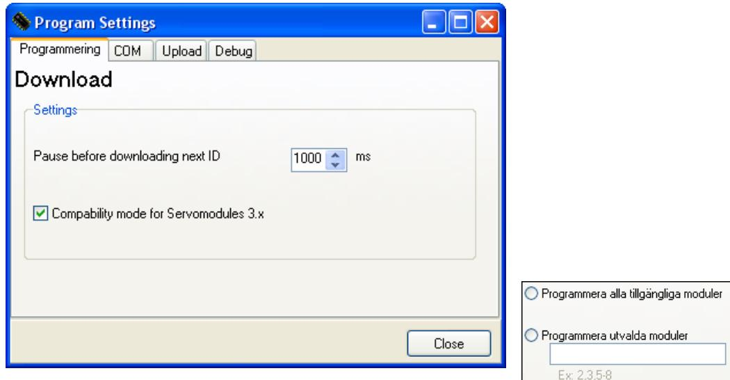
When programming more than one ID at the time, there is a pause time between the different ID:s. It's possible to change this pause time to optimize programming, or to raise the time if problems occur when programming.
