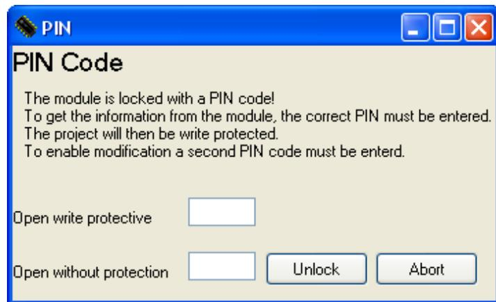
If the hardware module has been programmed with a PIN code, an upload will result in a dialog window opening. Here it's possible to upload the module to the project as Read-Only or upload the module to the project as normal, with no limitations.
