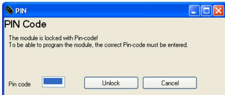
In those cases when the CanCom module has been programmed with the programming-PIN, will this dialog show. PIN code has to be entered to program the CanCom module again.
