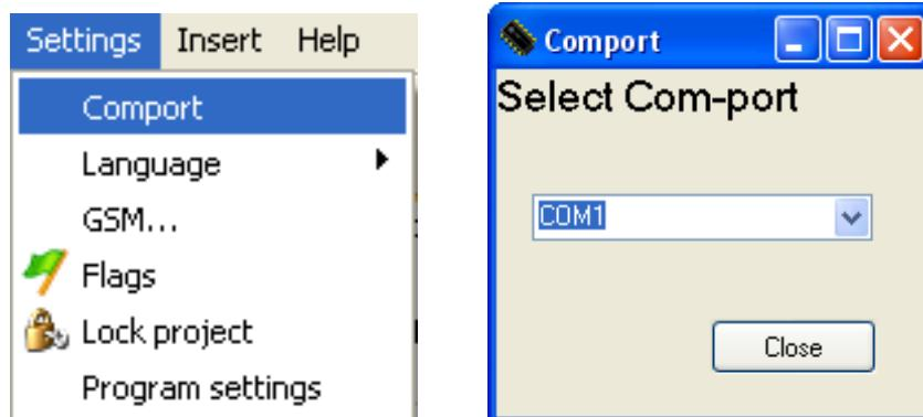
Select the serial port on which the CAN-interface is connected.
