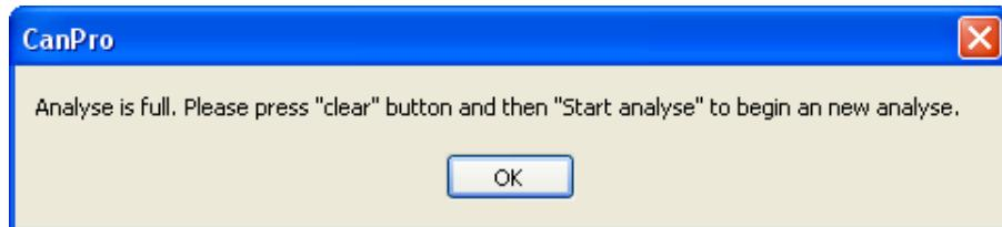
A log file can at most hold 19.000 log points. The logs are saved every 20 ms, for as many as 8 channels at the time. In other words, more channels equals lesser time before the log is full.
