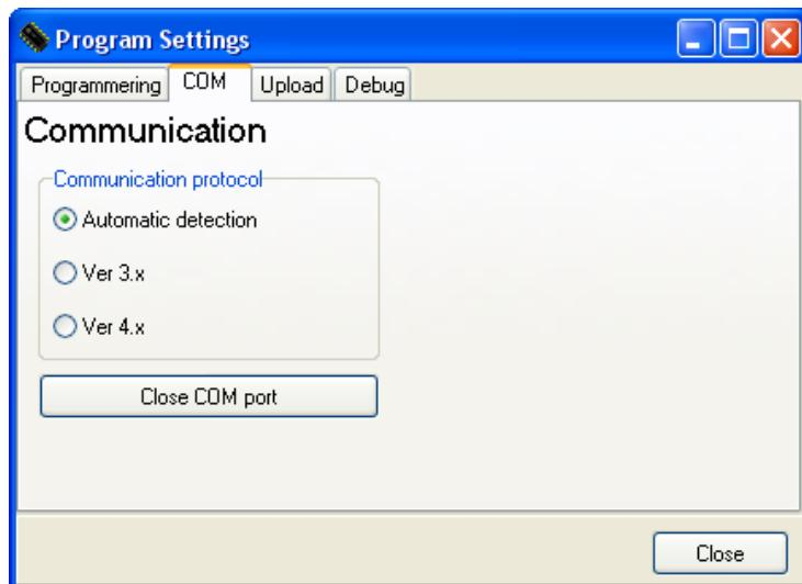
CanPro can be set in three different communication moods. This is due to backward capability with old hardware. If the radio button is set to automatic, the hardware version is detected and the appropriate algorithm is used. The two later radio buttons can lock the communication into ver3 or ver4 communication protocol. This could be used if problems occur when programming with unknown hardware.
